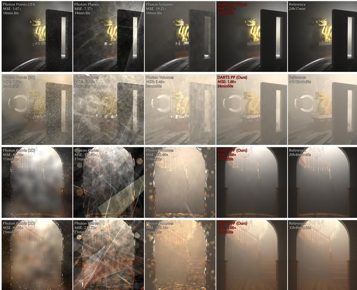
Fig. X. Comparison with other estimators proposed by Liu et al. [2022], mainly *transient photon planes* and *transient photon volumes*. Except for the image rendered by photon volumes in the second time point of the GLOSSY DRAGON scene (row 2, col 2), of which the MSE is lower than photon points method, all other cases are found to perform poorly. Therefore, these estimators are not included in our paper.
